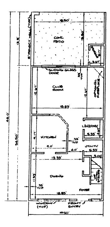
TYPICAL UNIT FLOOR PLAN
