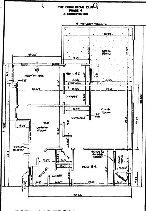
TYPICAL UNIT FLOOR PLAN
