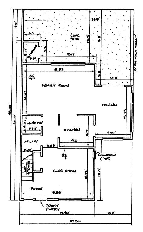
TYPICAL UNIT FLOOR PLAN
