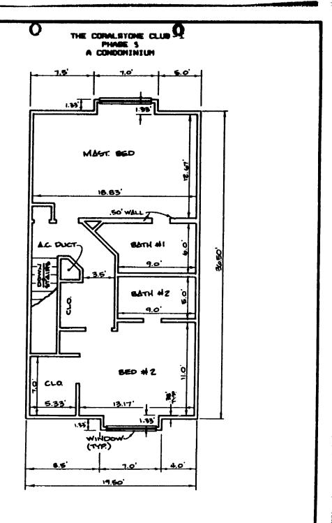
TYPICAL UNIT FLOOR PLAN
