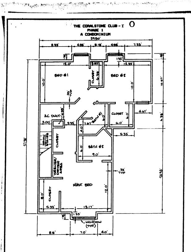
TYPICAL UNIT FLOOR PLAN
