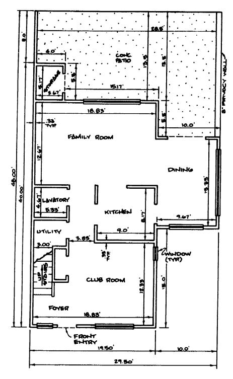
TYPICAL UNIT FLOOR PLAN
