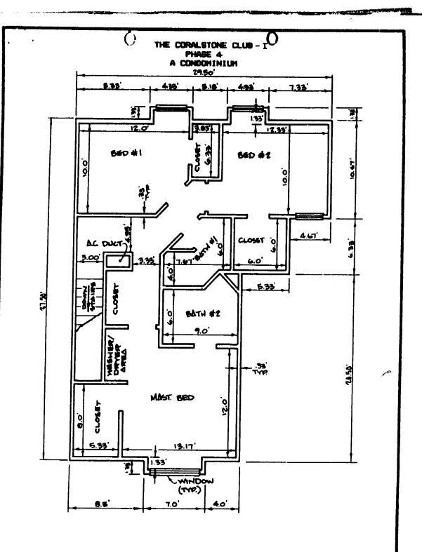
TYPICAL UNIT FLOOR PLAN
