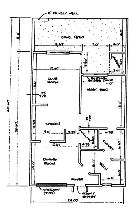
TYPICAL UNIT FLOOR PLAN
