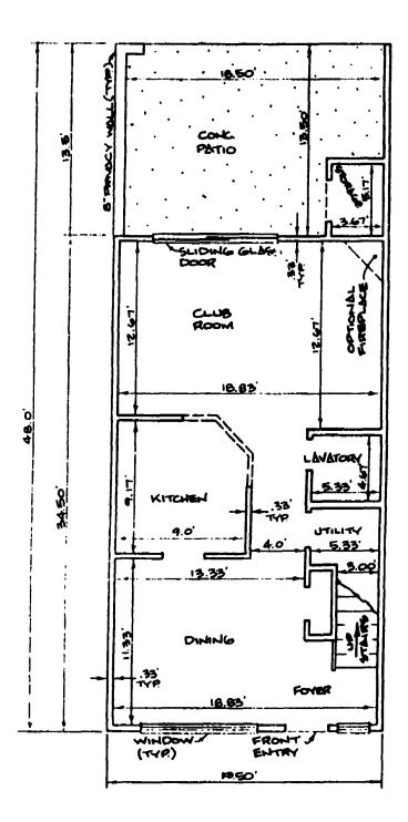
TYPICAL UNIT FLOOR PLAN
