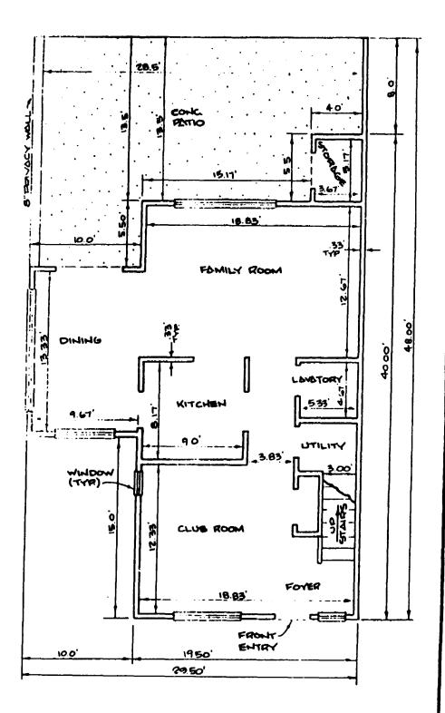
TYPICAL UNIT FLOOR PLAN
