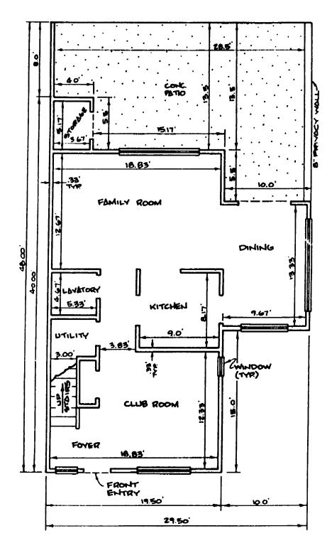
TYPICAL UNIT FLOOR PLAN
