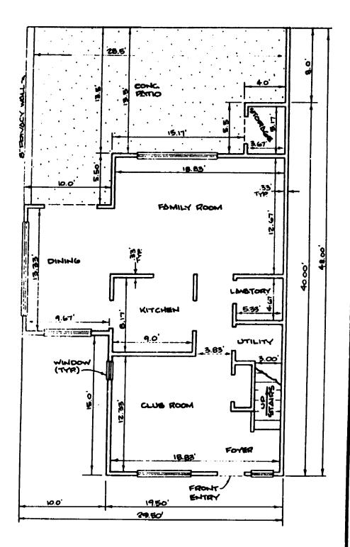
TYPICAL UNIT FLOOR PLAN
