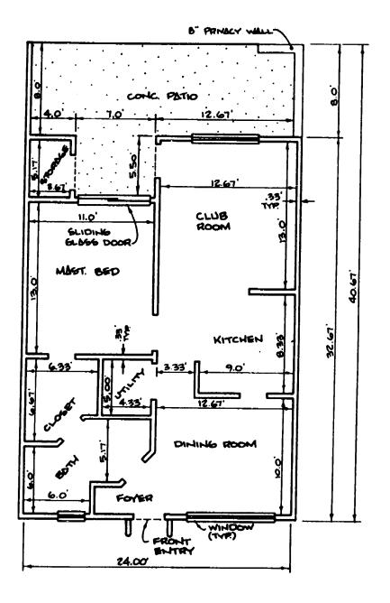
TYPICAL UNIT FLOOR PLAN
