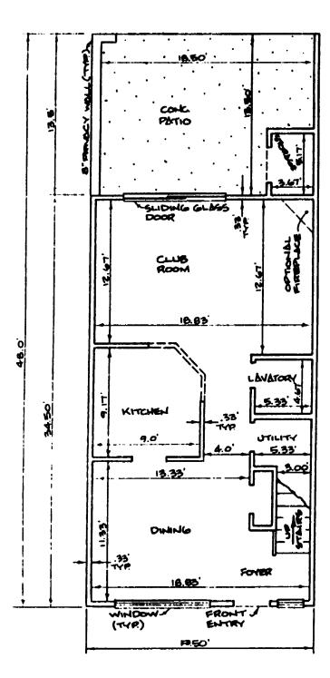
TYPICAL UNIT FLOOR PLAN
