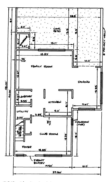
TYPICAL UNIT FLOOR PLAN
