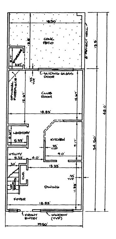
TYPICAL UNIT FLOOR PLAN
