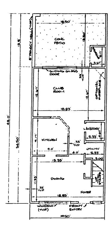
TYPICAL UNIT FLOOR PLAN
