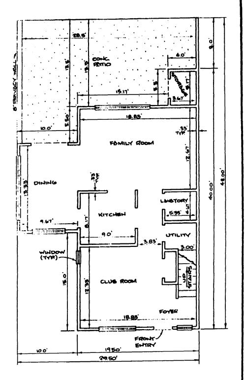
TYPICAL UNIT FLOOR PLAN
