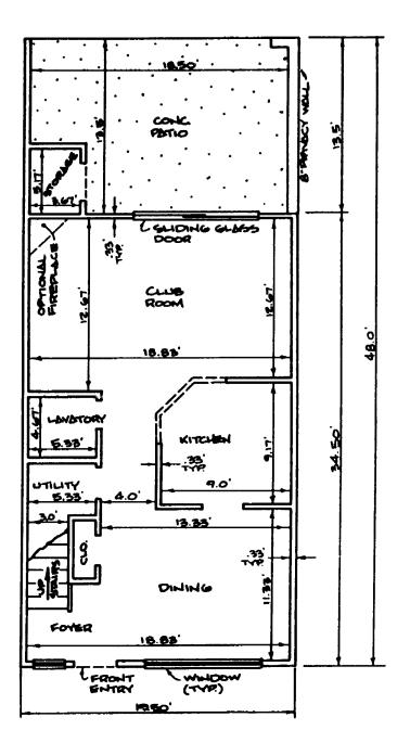
TYPICAL UNIT FLOOR PLAN
