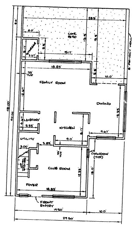
TYPICAL UNIT FLOOR PLAN
