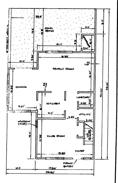
TYPICAL UNIT FLOOR PLAN
