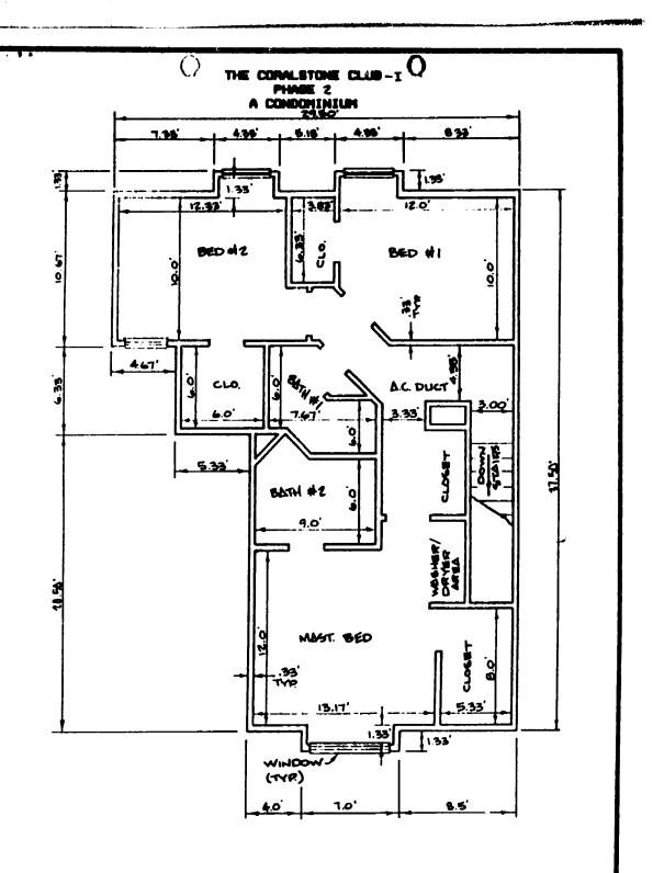
TYPICAL UNIT FLOOR PLAN
