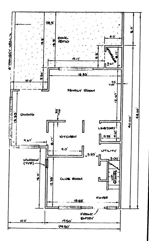
TYPICAL UNIT FLOOR PLAN
