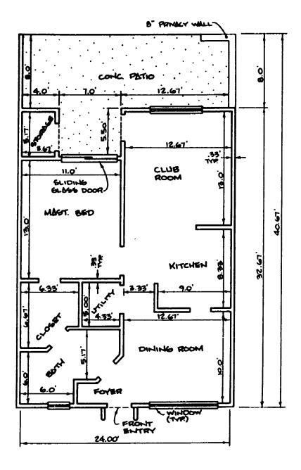
TYPICAL UNIT FLOOR PLAN
